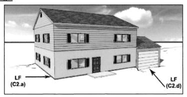
A garage attached to a residential structure or in an enclosed area below an elevated building may have the garage floor slab below the Base Flood Elevation (BFE). Because such a garage is an enclosed area below the BFE, openings are required either in the exterior walls of the garage or in the garage doors themselves.
