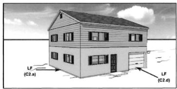
Enclosures are enclosed walled in areas below the *lowest floor of an elevated building*. Enclosures below the Base Flood Elevation (BFE) may only be used for **building access**, **vehicle parking**, **and storage**. Enclosed areas below the lowest floor must be adequately anchored, built using flood resistant building material, and any utilities or service facilities must be designed and/or located to prevent flood damage.
