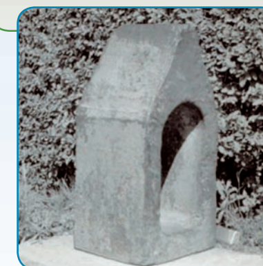
This nearly 500-pound hammer was used to forge at the Iron Works on the Little Pigeon River over 150 years ago. It is pictured here at the home of Robert Wear in the 1940s.
